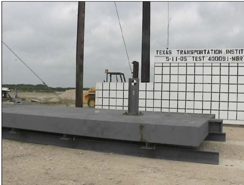
Crash barrier bolted to SPS Bridge Deck
